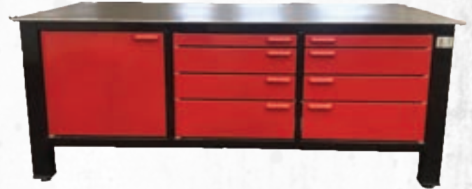
3BAY Double Wide with 3/8" plate steel top
